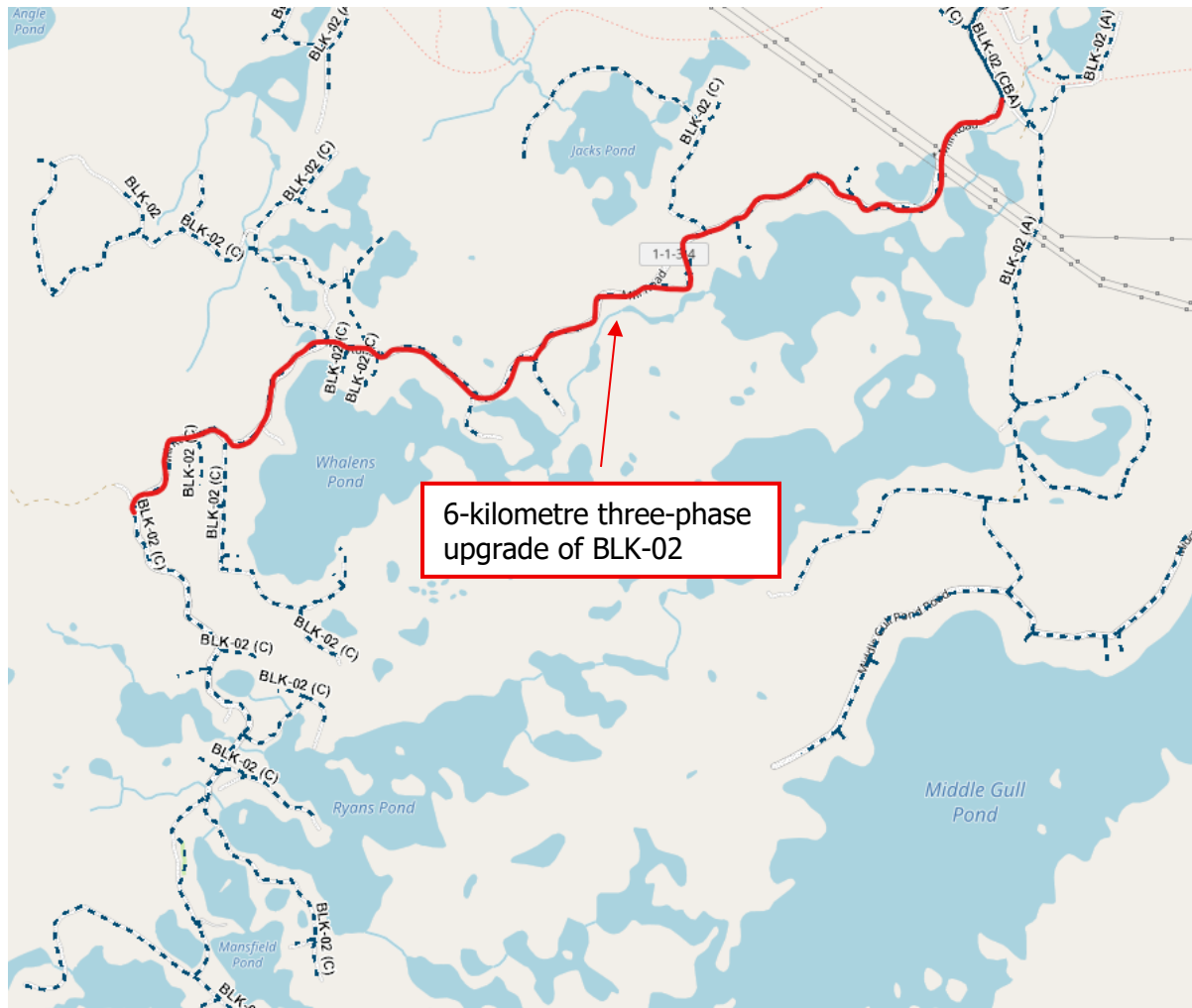
Figure 2 – Three-Phase Upgrade of Distribution Feeder BLK-02
