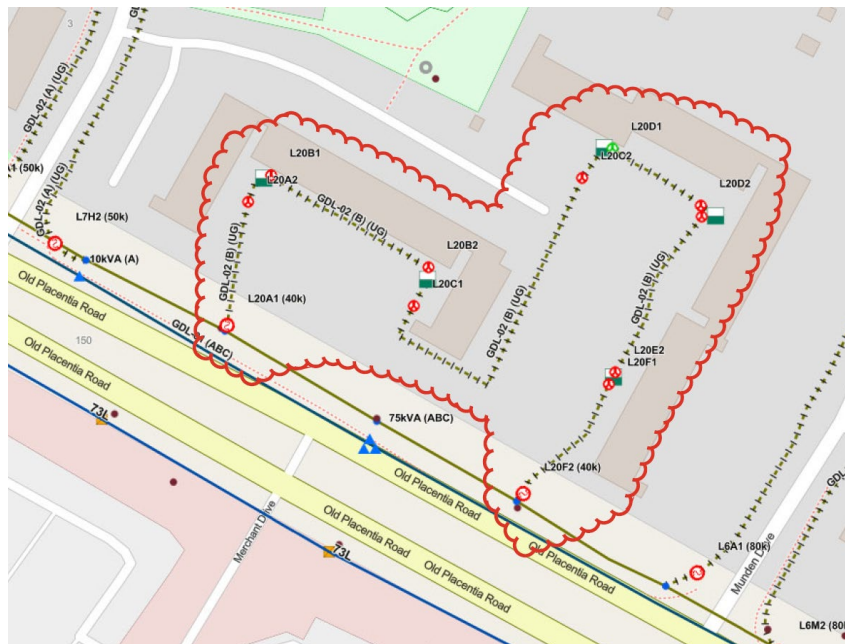
Figure 2 - Distribution Feeder GDL-02, Loop 20
